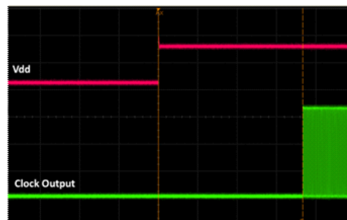
Figure 17. Startup Waveform vs. Vdd
