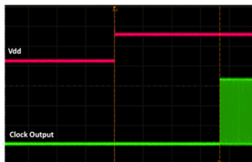
Figure 16. Startup Waveform vs. Vdd
